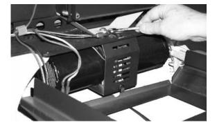
**12)** Before re-attaching the rear access panel, the valve wires and the fan wires need to be connected.
